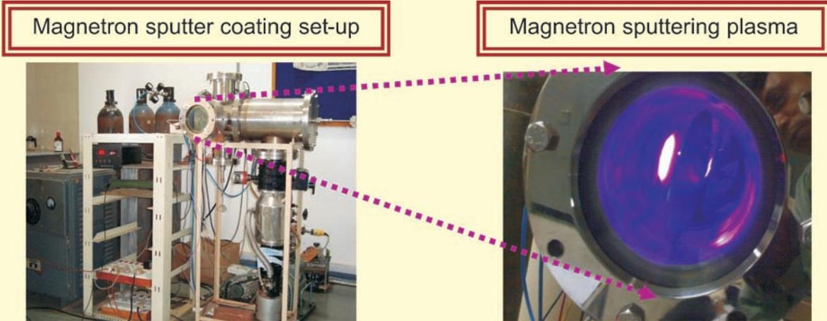
**Fig. 2:** Experimental set-up showing plasma during sputtering process.
