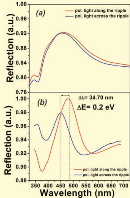
**Fig. 3:** Reflection of light polarized along and across the ripple direction showing LSPR (a) of non-ordered particles on a flat Si surface shown in Fig. 2(a); and (b) of ordered particles shown in Fig. 2(c).
