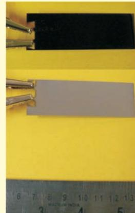
**Fig. 3:** Perfectly optically opaque and uniform carbon coating (top) and over that shining aluminum coating (bottom).
