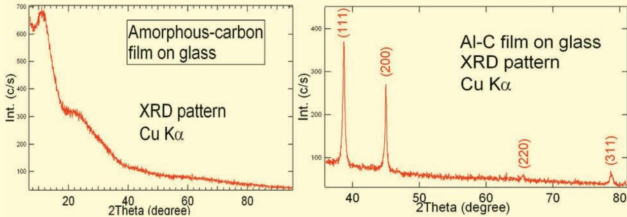
Fig. 4: XRD patterns of Aluminum (left) on bi-layer and amorphous carbon film (right)
