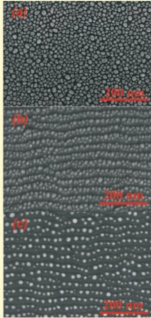
**Fig. 2:** SEM images of Ag nanoparticles grown (a) on a flat Si substrate at room temperature, (b) on a ripple patterned substrate at room temperature; and (c) on a ripple patterned substrate followed by annealing at 300°C for 60 minutes.
