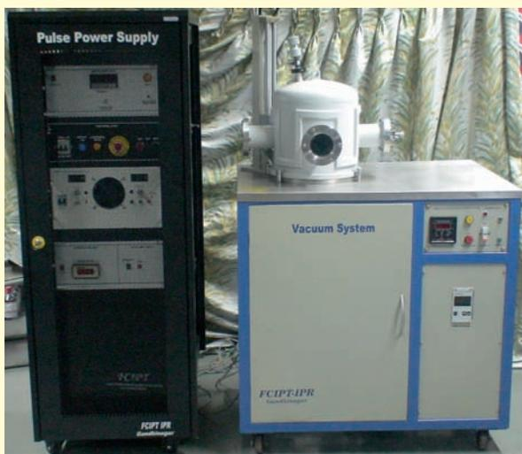
Photograph of the Pulsed glow discharge plasma System
