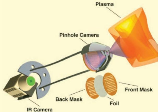
**Fig. 1:** Schematic picture of thin foil IR imaging bolometer (Reproduced from Ref. 1)
