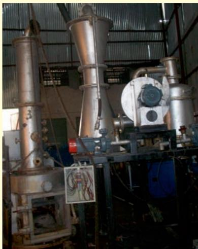
Photograph of the Plasma Pyrolysis system that was installed at Doon hospital, Dehradun
