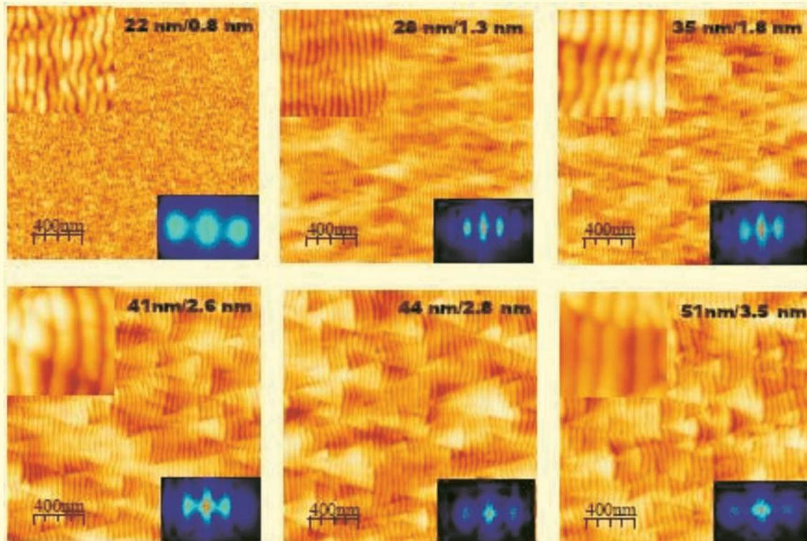
**Fig. 1:** AFM images of ripple patterns with different periodicity produced by 500 eV  $Ar^+$  ion irradiation at  $67^\circ$  incidence on Si substrate with fluences of  $10^{16-19} \text{ cm}^{-2}$ . The corresponding wavelength and roughness (rms) values are mentioned on each image. Zoomed portion and FFT shown in inset reflect the quality of ripples.
