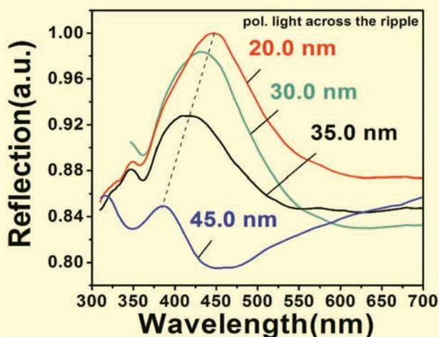
**Fig. 4:** Reflection of light polarized across the ripples showing a LSPR which is red shifted with decreasing ripple wavelength from 45 nm to 20 nm.
