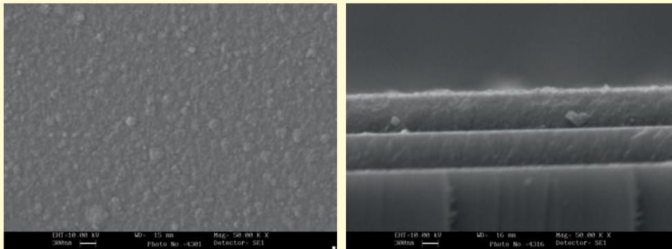
Fig. 5: SEM micrograph of the surface and cross section of the bi-layer.
