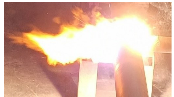
Figure 2. Plasma arc using graphite electrodes
