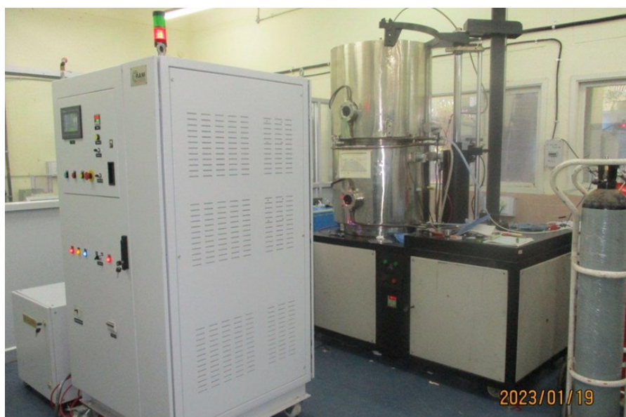
Figure 3: Picture of pulsed HV DC power supply integrated with Plasma Nitriding system at IGCAR Kalpakkam
