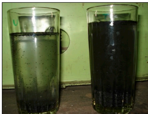
Figure 4: Side view of glasses is showing the untreated floated powder (Left) and dissolved treated powder (Right)
