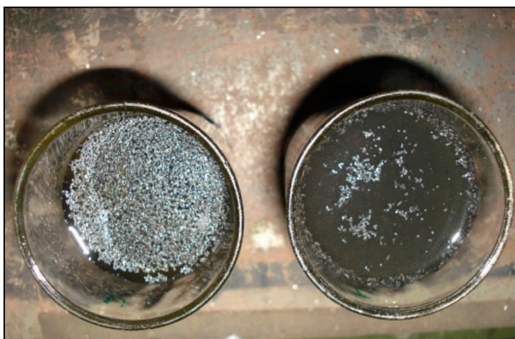
Figure 3: Top view showing floated untreated carbon powder (Left) and treated carbon powder is settled at the bottom (Right)
