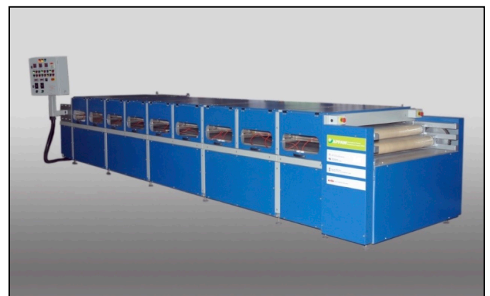
Figure 2: Atmospheric pressure air plasma system for Angora wool treatment
