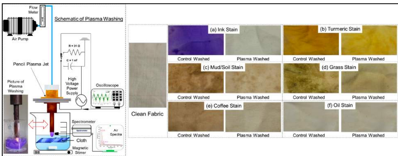
Fig.1: Schematic of plasma washing using dielectric barrier discharge pencil plasma jet. Visual appearance of fabric after control and plasma washing (a) Ink stain, (b) Turmeric stain, (c) Mud/Soil stain, (d) Grass stain, (e) Coffee stain, (f) Oil stain [3]
