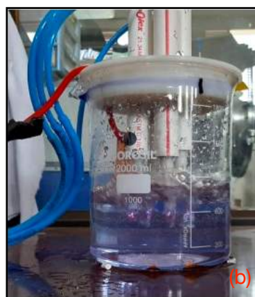
Fig.1: Atmospheric pressure plasma jets (a) schematic of the experimental setup (b) actual plasma jets in contact with water.
