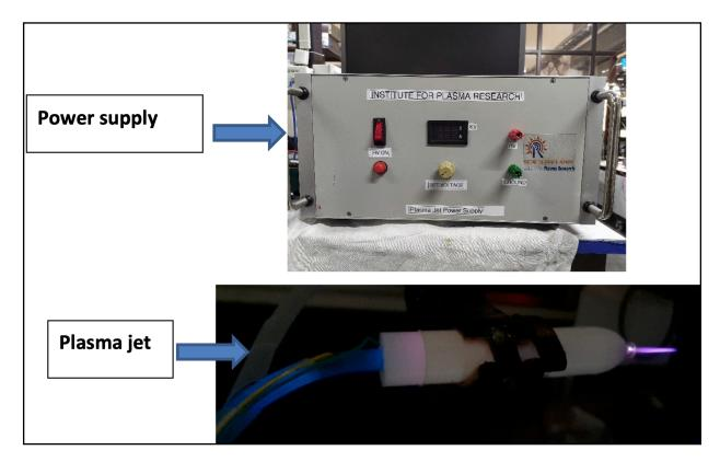
The Atmospheric pressure plasma jet and power supply developed at FCIPT and installed at BIT, Mesra, Jaipur
