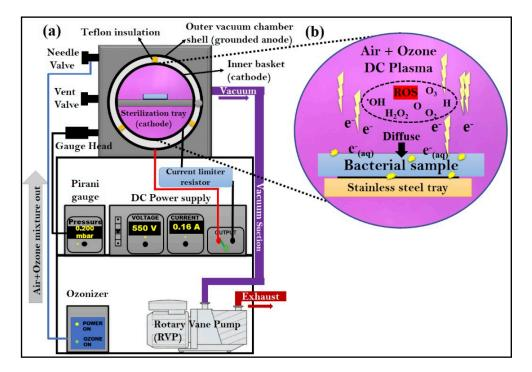
Figure 1: (a) Schematic diagram of Plasma sterilization system, and (b) Broad view of plasma-bacterial suspension interactions and ROS generation
